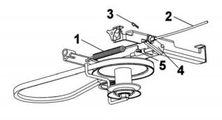
Install the manual clutch cable
