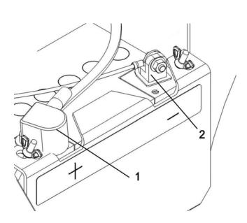
Connect the relay wires to the battery
