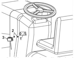
Install the support and control box for the winch
