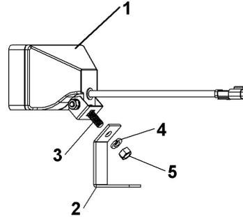
Drill a hole with a 11/32" bit at the appropriate place to install the light.
