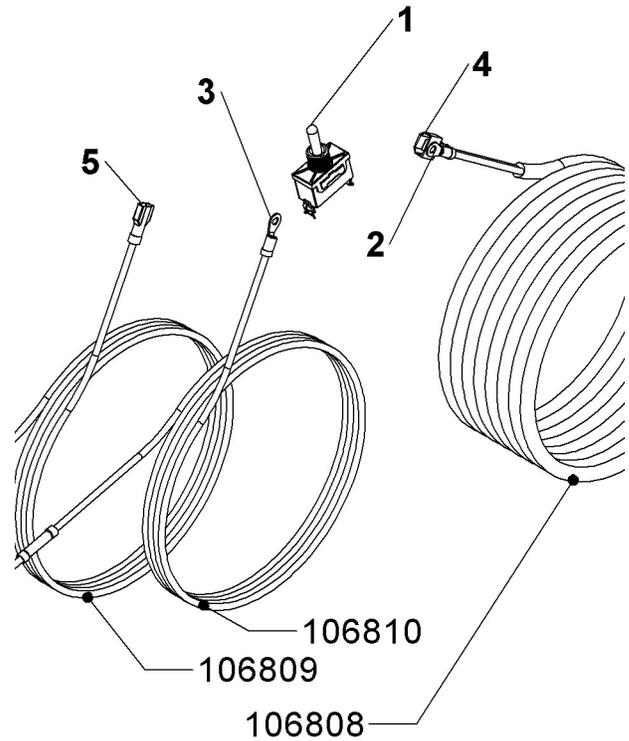
Drill a  $\varnothing 1/2''$  hole in the appropriate place in the dashbord. Set the switch (item 1) into the hole and secure it in place with the cap (item 2).
