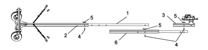
This extension for universal subframe allows the installation of an accessory on a vehicle that is longer than most. The option inserted in the original subframe will add 33 in. to the length of the subframe. To choose the right adjustment:
